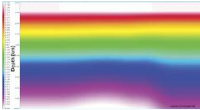
Figure 1. Initial depth-imaging velocity model.
