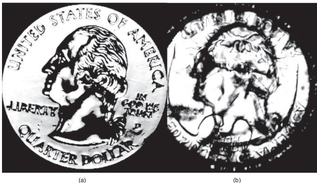
Fig. 2—Scanning acoustic image of a USD 0.25 coin: (a) shows a surface image and (b) was obtained by focussing approximately 2 mm (300 ns) into the coin.
